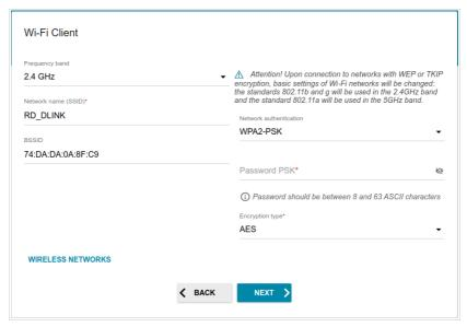
If you connect to a hidden network, select the band where the hidden network operates from the **Frequency band** list and enter the network name in the **Network name (SSID)** field. Then select a needed value from the **Network authentication** list and then, if needed, enter the password in the relevant field.
