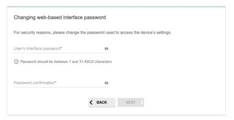
Remember or write down the new password for the administrator account. In case of losing the new password, you can access the settings of the router only after restoring the factory default settings via the hardware RST/WPS button. This procedure wipes out all settings that you have configured for your router.
