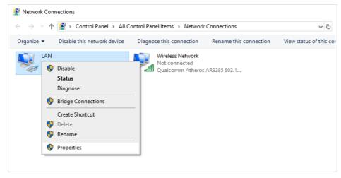
In the Local Area Connection Properties window, on the Networking tab, select the Internet Protocol Version 4 (TCP/IPv4) line. Click the Properties button.  Make sure that the Obtain an IP address automatically and Obtain DNS server address automatically choices of the radio buttons are selected. Click the OK button.
