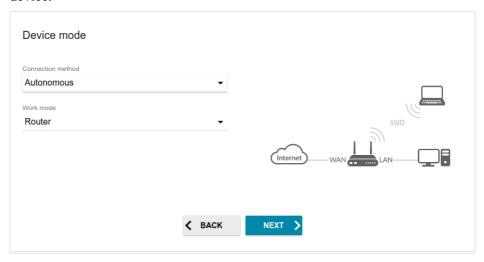
In order to connect your device to a wireless ISP (WISP), on the **Device** mode page, from the **Connection method** list, select the **Autonomous** value. Then from the **Work mode** list, select the **WISP Repeater** value. In this mode you can connect your device to another access point, configure a WAN connection, set your own settings for the wireless network in the 2.4GHz and 5GHz bands, and set your own password for access to the webbased interface of the device.
