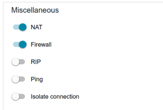
Figure 57. The page for creating a new Static IPv4 connection. The Miscellaneous section.
