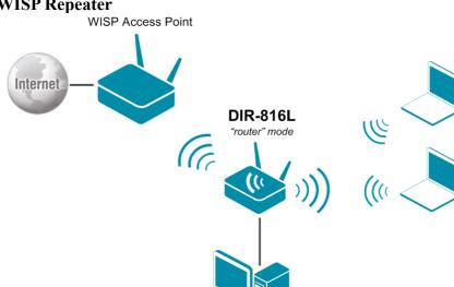
The DIR-816L device in the "router" mode is connected to a WISP access point via wireless connection. Computers connect to DIR-816L via wireless or wired connection. It is necessary to configure the same channel of the wireless connection for DIR-816L and the WISP access point. Other parameters of the wireless network of DIR-816L do not depend upon the settings of the WISP access point. In addition, it is necessary to configure a WAN connection for DIR-816L.
