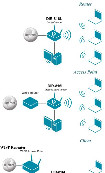
The DIR-816L device in the "router" mode is connected to a private Ethernet line or to a cable or DSL modem. Computers connect to DIR-816L via wireless or wired connection.
