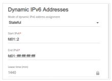
6. After specifying the needed parameters on the **Connections Setup** / **LAN** page, click the **APPLY** button.
