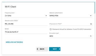
If you connect to a hidden network, select the band where the hidden network operates from the **Frequency band** list and enter the network name in the **Network name (SSID)** field. Then select a needed value from the **Network authentication** list and then, if needed, enter the password in the relevant field.
