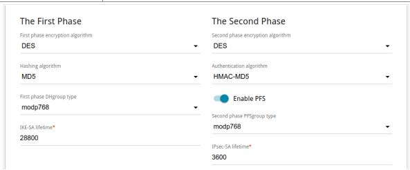
Figure 125. The page for adding an IPsec tunnel. The First Phase / The Second Phase sections.
