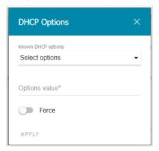
Figure 81. Configuring the local interface. The **IPv4** tab. The window for configuring a DHCP option. In the opened window, you can specify the following parameters:
