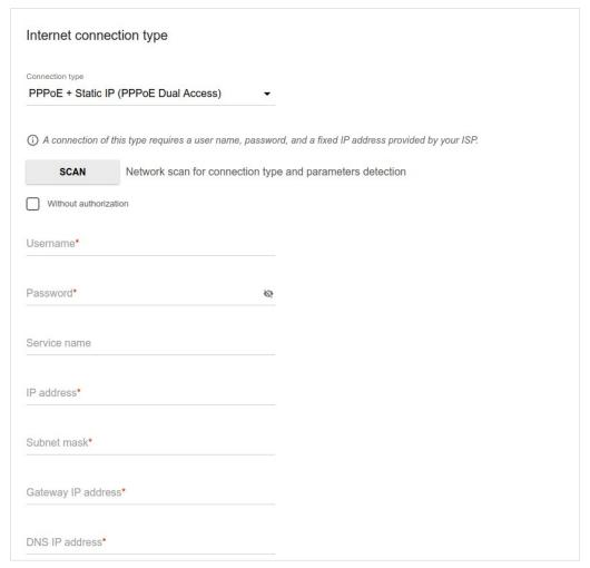
Figure 43. The page for configuring PPPoE + Static IP (PPPoE Dual Access) WAN connection.
