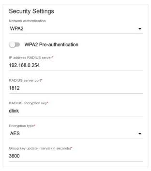
Figure 92. The WPA2 value is selected from the Network authentication drop-down list.
