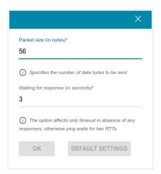
Figure 140. The System / Ping page. The additional settings window.
