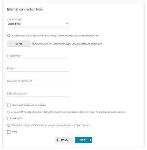
Figure 41. The page for configuring Static IPv6 WAN connection.
