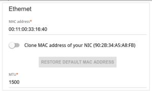
Figure 75. The page for creating a new **PPPoE IPv6** connection. The **Ethernet** section.
