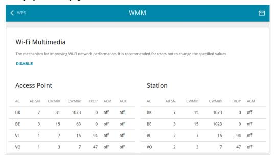
Figure 95. The page for configuring the WMM function.
