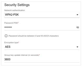
Figure 91. The WPA2-PSK value is selected from the Network authentication drop-down list.
