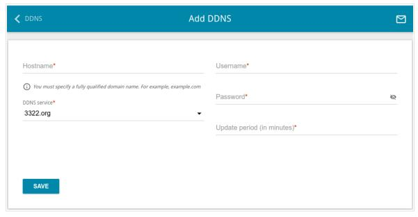
Figure 109. The page for adding a DDNS service.
