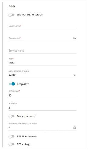
Figure 71. The page for creating a new **PPPoE** connection. The **PPP** section.
