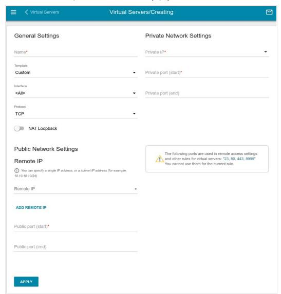
Figure 130. The page for adding a virtual server.
