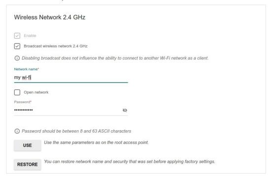
Figure 46. The page for configuring the wireless network.
