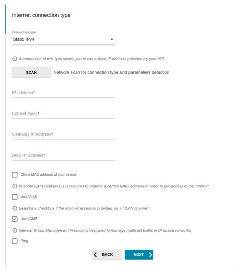
Figure 40. The page for configuring Static IPv4 WAN connection.
