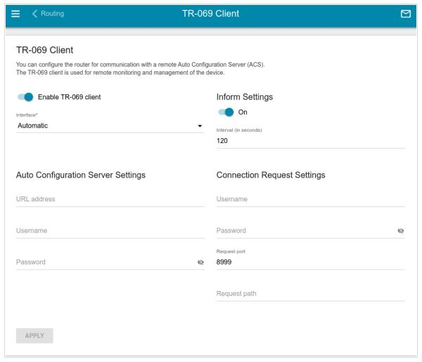
Figure 115. The page for configuring the TR-069 client.
