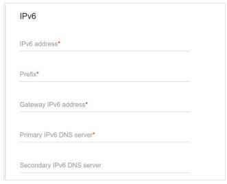
Figure 68. The page for creating a new **Static IPv6** connection. The **IPv6** section.
