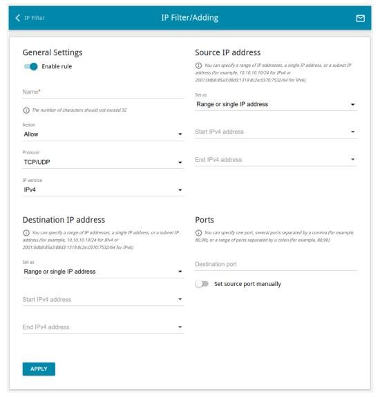
Figure 128. The page for adding a rule for IP filtering.
