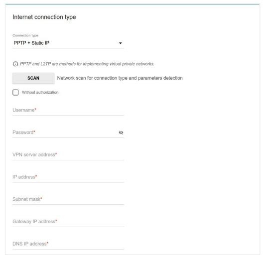
Figure 45. The page for configuring PPTP + Static IP WAN connection.
