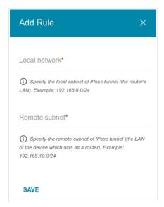
Figure 126. The page for adding an IPsec tunnel. The window for adding a tunneled network. In the opened window, you can specify the following parameters:
