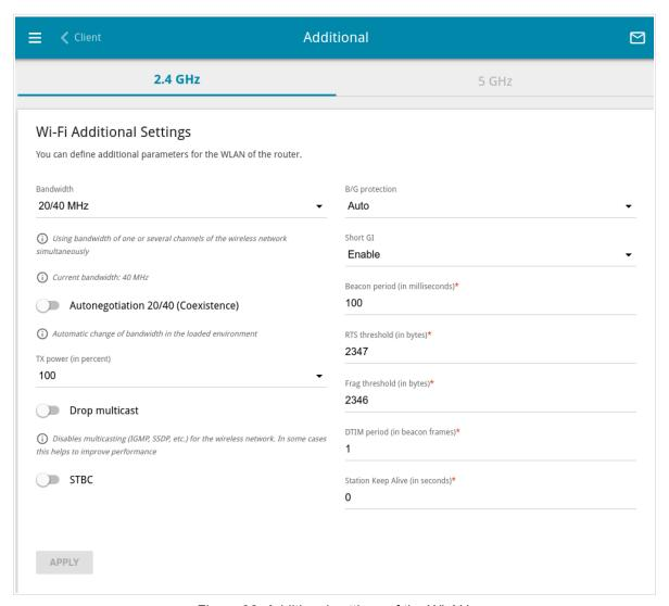
Figure 98. Additional settings of the WLAN.
