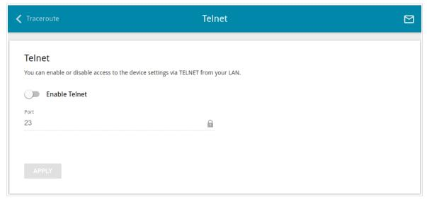
Figure 143. The System / Telnet page.
