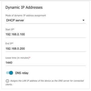
Figure 79. Configuring the local interface. The **IPv4** tab. The **Dynamic IP Addresses** section.
