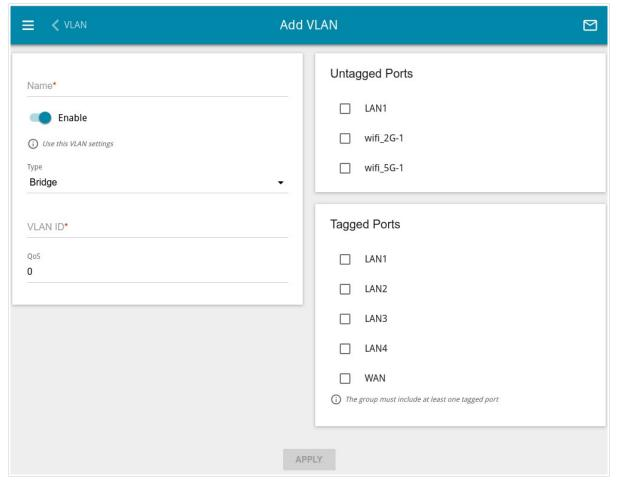
Figure 103. The page for adding a VLAN.
