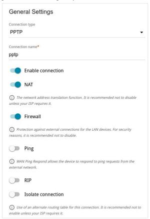
Figure 72. The page for creating a new **PPTP** connection. The **General Settings** section.
