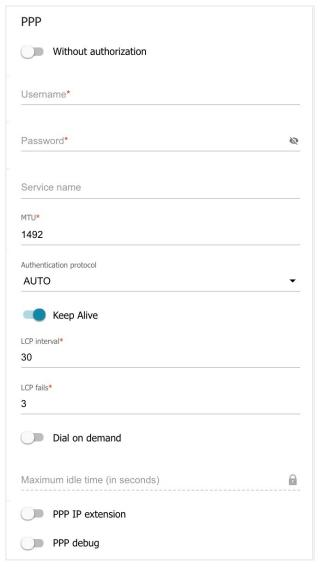
Figure 76. The page for creating a new **PPPoE IPv6** connection. The **PPP** section.
