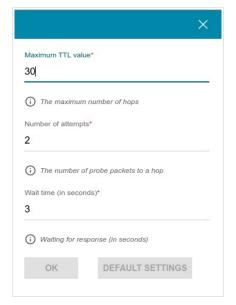
Figure 142. The System / Traceroute page. The additional settings window.
