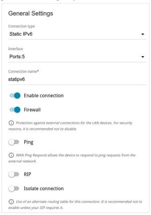
Figure 66. The page for creating a new Static IPv6 connection. The General Settings section.
