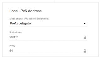
Figure 83. Configuring the local interface. The IPv6 tab. The Local IPv6 Address section.
