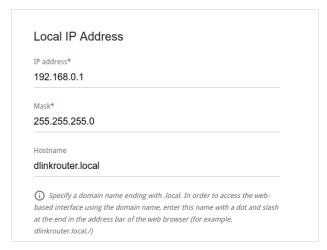
Figure 78. Configuring the local interface. The IPv4 tab. The Local IP Address section.
