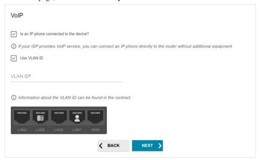
Figure 49. The page for selecting a LAN port to connect an VoIP phone.
