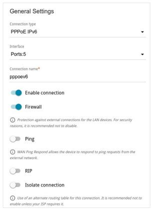
Figure 74. The page for creating a new PPPoE IPv6 connection. The General Settings section.
