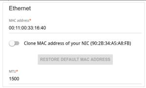
Figure 67. The page for creating a new **Static IPv6** connection. The **Ethernet** section.
