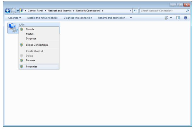
Figure 5. The **Network Connections** window.
