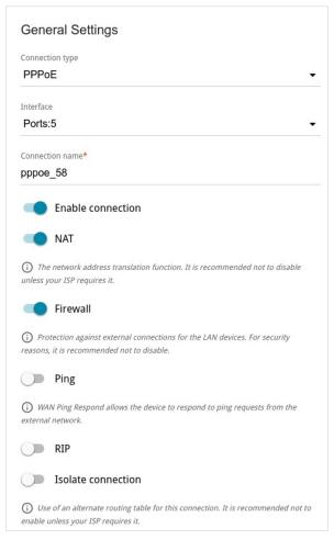
Figure 69. The page for creating a new PPPoE connection. The General Settings section.
