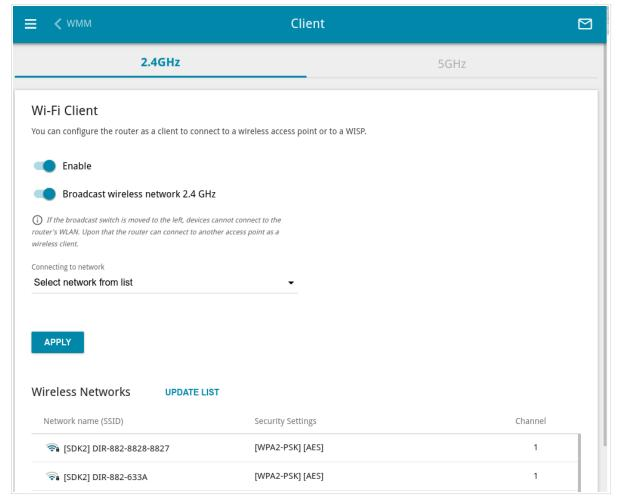
Figure 97. The page for configuring the client mode.
