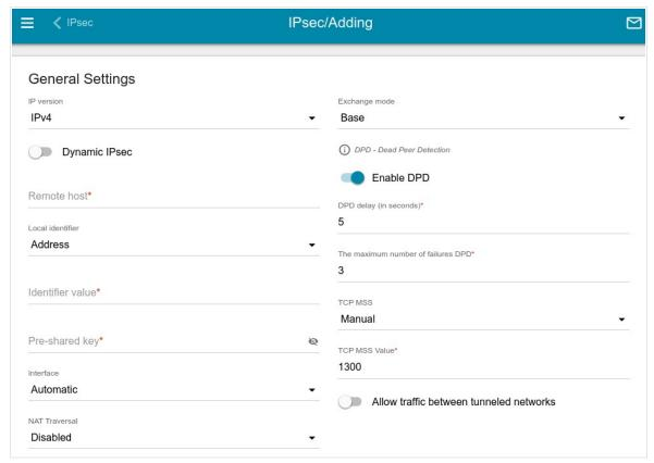
Figure 124. The page for adding an IPsec tunnel. The General Settings section.
