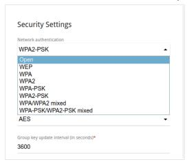
Figure 89. Network authentication types supported by the router.
