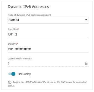
Figure 84. Configuring the local interface. The IPv6 tab. The Dynamic IPv6 Addresses section.
