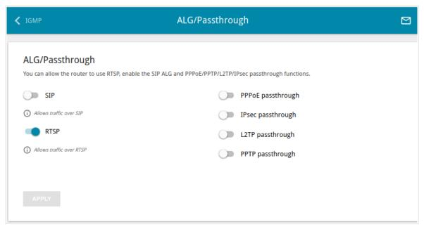
Figure 122. The Advanced / ALG/Passthrough page.
