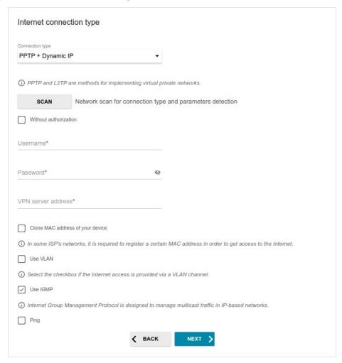
Figure 44. The page for configuring PPTP + Dynamic IP WAN connection.
