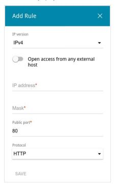
Figure 117. The window for adding a rule for remote management.
