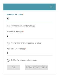
Figure 142. The **Management / Diagnostics / Traceroute** page. The additional settings window. In the opened window, you can specify the following parameters:
