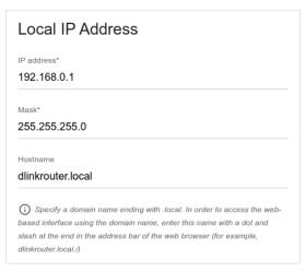
Figure 82. Configuring the local interface. The IPv4 tab. The Local IP Address section.
