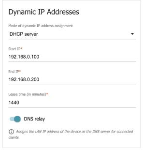
Figure 83. Configuring the local interface. The IPv4 tab. The Dynamic IP Addresses section.
