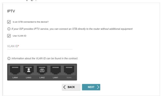
Figure 50. The page for selecting a LAN port to connect an IPTV set-top box.
