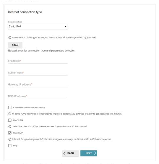
Figure 42. The page for configuring Static IPv4 WAN connection.
