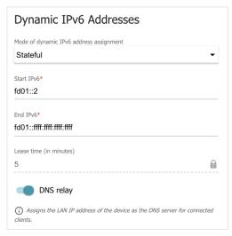
Figure 88. Configuring the local interface. The **IPv6** tab. The **Dynamic IPv6 Addresses** section.
