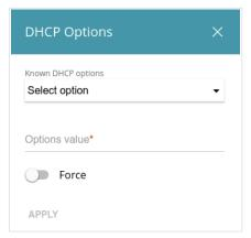
Figure 85. Configuring the local interface. The **IPv4** tab. The window for configuring a DHCP option. In the opened window, you can specify the following parameters:
