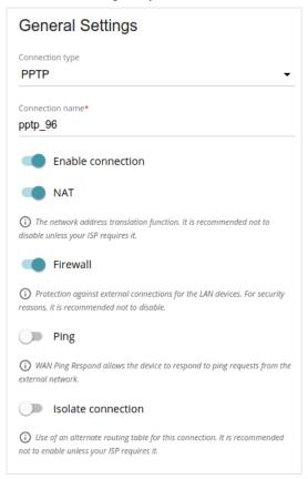
Figure 65. The page for creating a new PPTP connection. The General Settings section.
