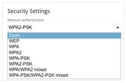
Figure 78. Network authentication types supported by the router.
