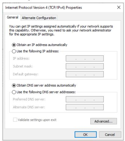
Figure 12. The Internet Protocol Version 4 (TCP/IPv4) Properties window.
