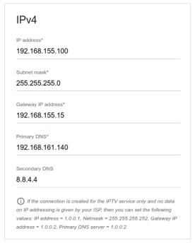
Figure 58. The page for creating a new Static IPv4 connection. The IPv4 section.
