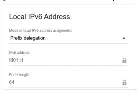
Figure 87. Configuring the local interface. The IPv6 tab. The Local IPv6 Address section.
