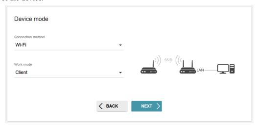
Figure 39. Selecting an operation mode. The Client mode.
