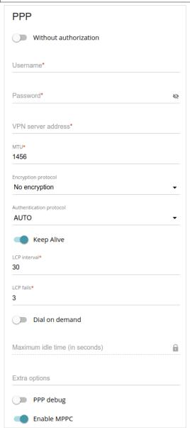
Figure 66. The page for creating a new **PPTP** connection. The **PPP** section.
