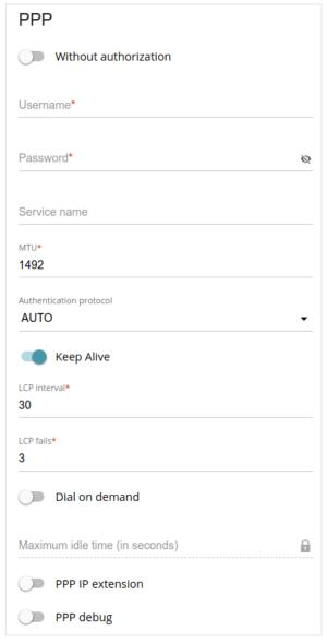
Figure 69. The page for creating a new **PPPoE IPv6** connection. The **PPP** section.
