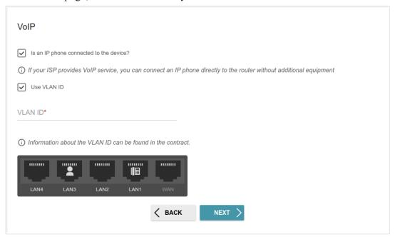
Figure 51. The page for selecting a LAN port to connect an VoIP phone.
