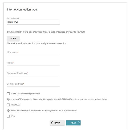
Figure 43. The page for configuring Static IPv6 WAN connection.
