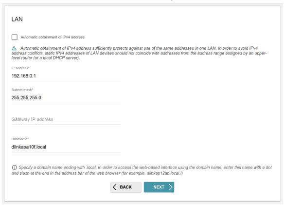
Figure 40. The page for changing the LAN IPv4 address.
