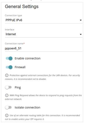
Figure 67. The page for creating a new PPPoE IPv6 connection. The General Settings section.
