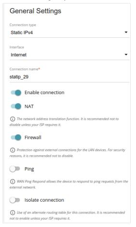
Figure 56. The page for creating a new Static IPv4 connection. The General Settings section.
