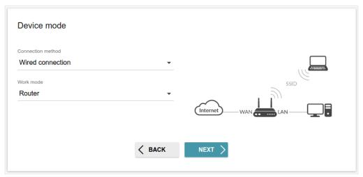
Figure 35. Selecting an operation mode. The Router mode.
