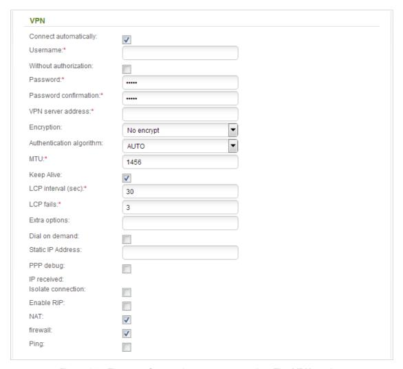
Figure 115. The page for creating a new connection. The **VPN** section.
