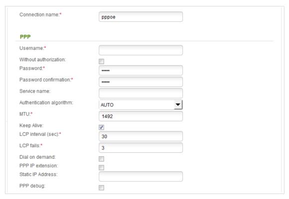
Figure 50. Configuring PPPoE + Dynamic IP WAN connection. The expert settings mode. The **PPP** section.
