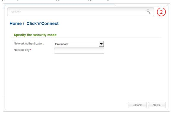
Figure 73. Selecting a security mode for the wireless network.
