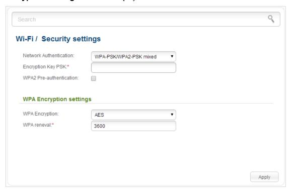
Figure 127. The **WPA-PSK/WPA2-PSK mixed** value is selected from the **Network Authentication** drop-down list.
