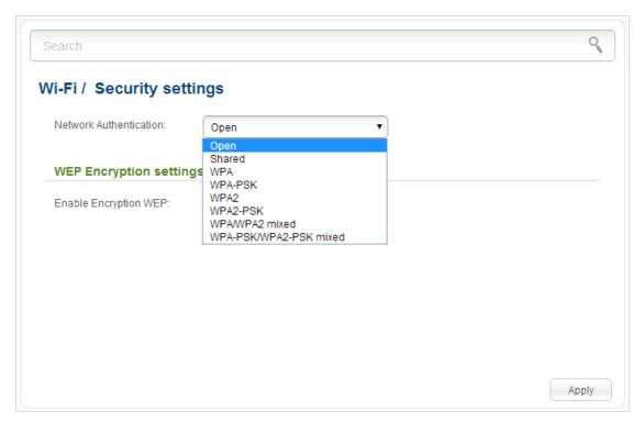
Figure 125. Network authentication types supported by the router.
