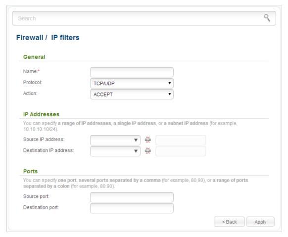
Figure 145. The page for adding a rule for IP filtering.
