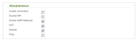
Figure 44. Configuring PPPoE + Static IP WAN connection. The expert settings mode.
