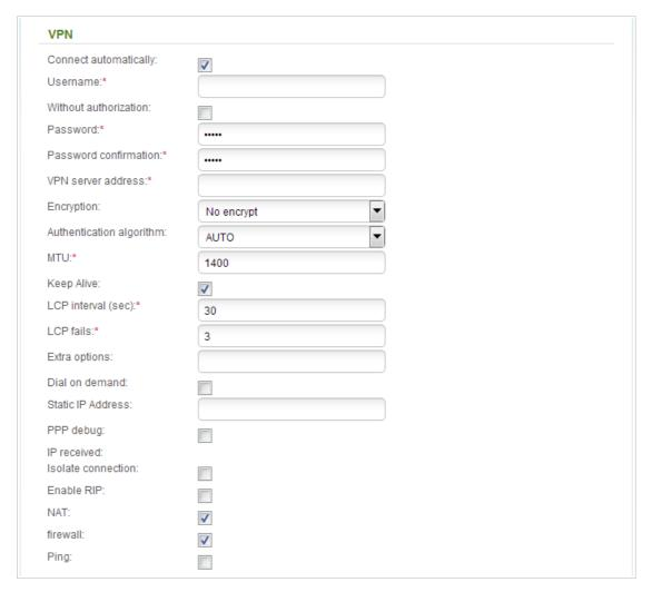
Figure 111. The page for creating a new connection. The **VPN** section.
