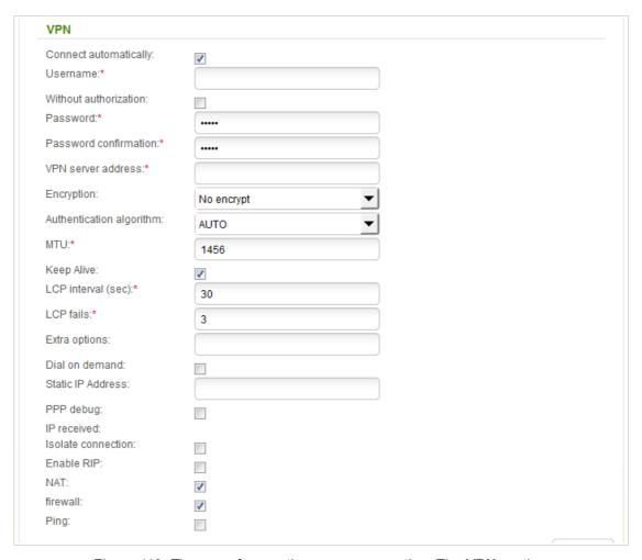
Figure 119. The page for creating a new connection. The VPN section.
