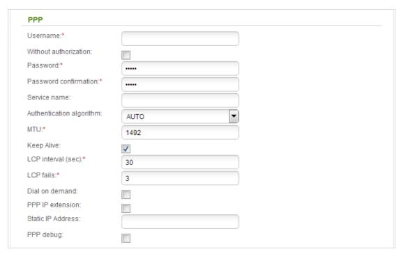
Figure 102. The page for creating a new connection. The PPP section.
