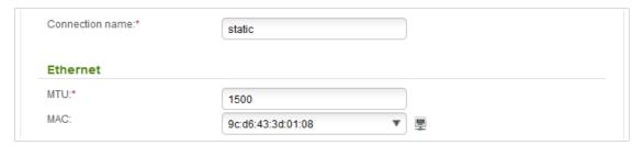
Figure 30. Configuring Static IP WAN connection. The expert settings mode. The **Ethernet** section.
