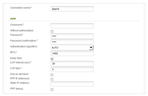
Figure 43. Configuring PPPoE + Static IP WAN connection. The expert settings mode. The **PPP** section.
