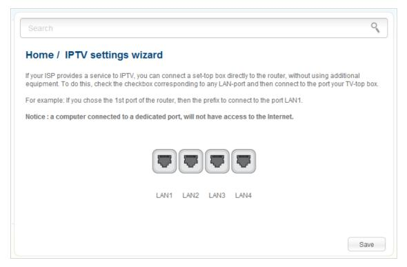
Figure 79. The page for selecting a LAN port to connect an IPTV set-top box.
