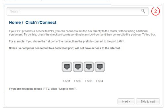
Figure 74. Selecting a LAN port to connect an IPTV set-top box.
