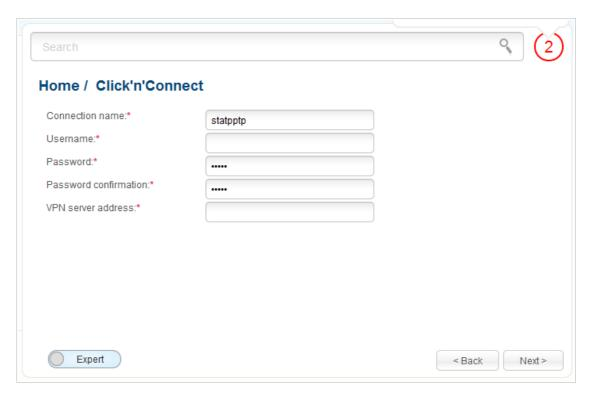
Figure 60. Configuring PPTP + Static IP WAN connection.
