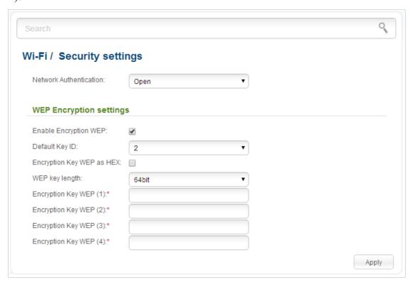
Figure 126. The Open value is selected from the Network Authentication drop-down list.
