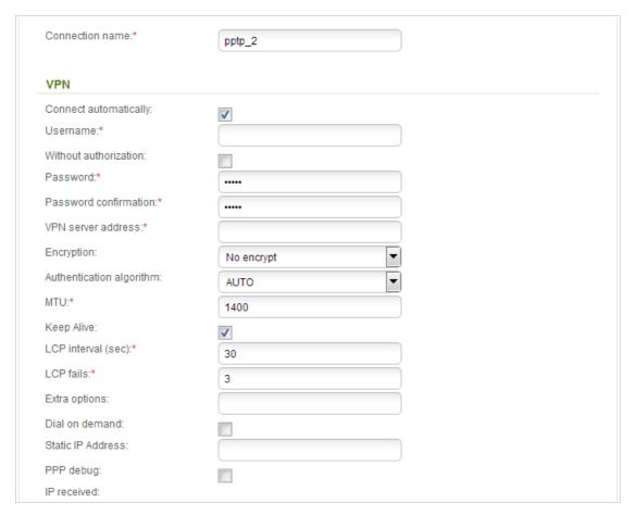
Figure 53. Configuring PPTP WAN connection. The expert settings mode. The VPN section.
