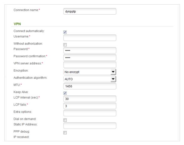
Figure 68. Configuring PPTP + Dynamic IP WAN connection. The expert settings mode. The **VPN** section.
