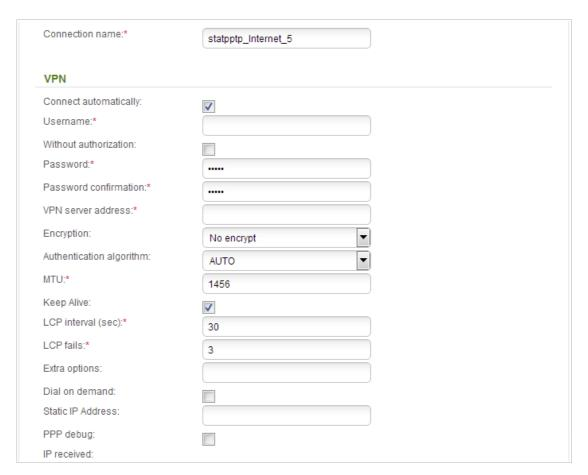
Figure 61. Configuring PPTP + Static IP WAN connection. The expert settings mode. The **VPN** section.
