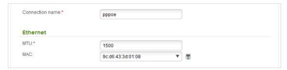
Figure 26. Configuring PPPoE WAN connection. The expert settings mode. The **Ethernet** section.
