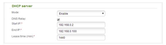
Figure 121. The section for configuring the DHCP server.
