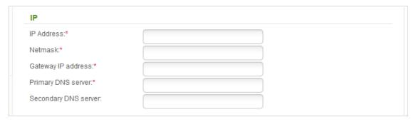
Figure 31. Configuring Static IP WAN connection. The expert settings mode. The IP section.
