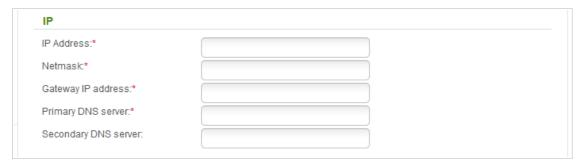
Figure 39. Configuring PPPoE + Static IP WAN connection. The expert settings mode. The IP section.
