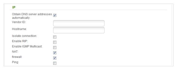
Figure 118. The page for creating a new connection. The **IP** section.
