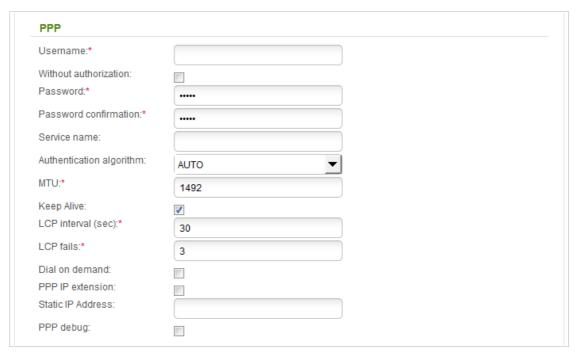
Figure 88. The page for creating a new connection. The **PPP** section.
