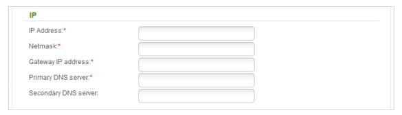
Figure 57. Configuring PPTP + Static IP WAN connection. The expert settings mode. The **IP** section.
