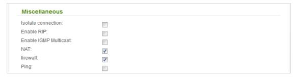
Figure 36. Configuring Dynamic IP WAN connection. The expert settings mode. The Miscellaneous section.
