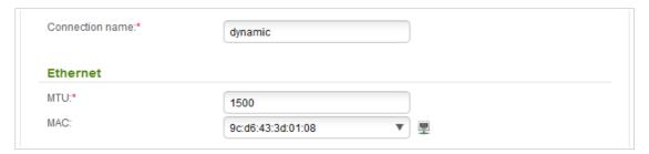
Figure 34. Configuring Dynamic IP WAN connection. The expert settings mode. The **Ethernet** section.
