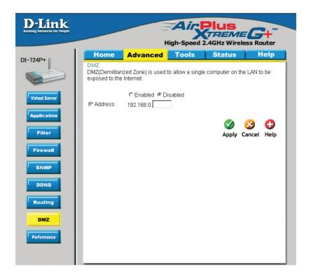
If you have a client PC that cannot run Internet applications properly from behind the DI-724P+, then you can set the client up for unrestricted Internet access. It allows a computer to be exposed to the Internet. This feature is useful for gaming purposes. Enter the IP address of the internal computer that will be the DMZ host. Adding a client to the DMZ (Demilitarized Zone) may expose your local network to a variety of security risks, so only use this option as a last resort.
