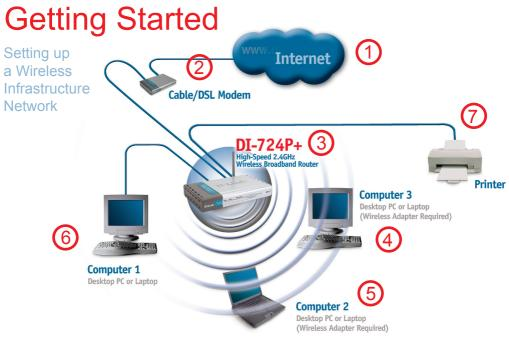
Please remember that D-Link AirPlus Xtreme G+ wireless devices are pre-configured to connect together, right out of the box, with their default settings. For a typical wireless setup at home (as shown above), please do the following:
