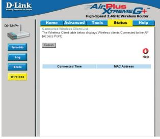
The wireless client table displays a list of current connected wireless clients. This table also displays the connection time and MAC address of the connected wireless client.
