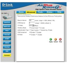
Beacon Interval-Beacons are packets sent by an Access Point to synchronize a wireless network. Specify a value. 100 is the default setting and is recommended.
