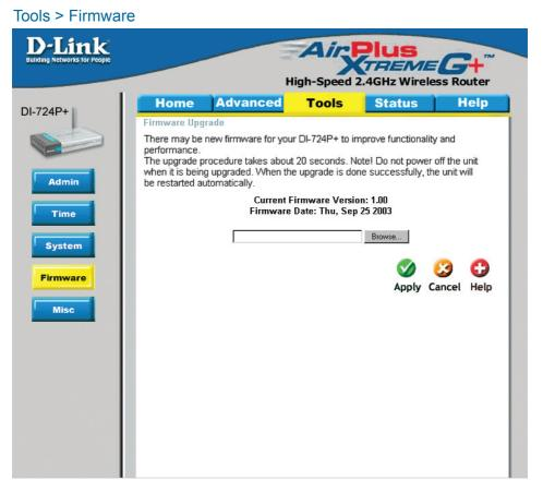
You can upgrade the firmware of the Router here. Make sure the firmware you want to use is on the local hard drive of the computer. Click on Browse to browse the local hard drive and locate the firmware to be used for the update. Please check the D-Link support site for firmware updates at http://support.dlink.com or global websites. You can download firmware upgrades to your hard drive from the D-Link support site.
